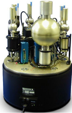
ROSPEC Neutron Spectrometer, a NATO-standard used at research facilities around the world
