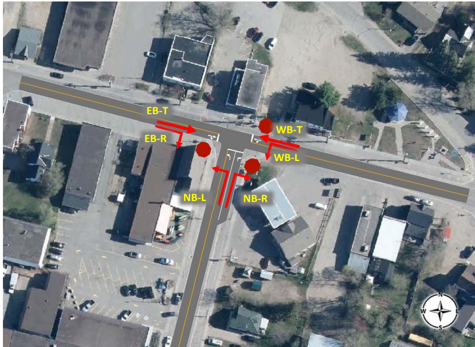
Figure 5.1 Test Scenario Layout of Barry's Bay Intersection
