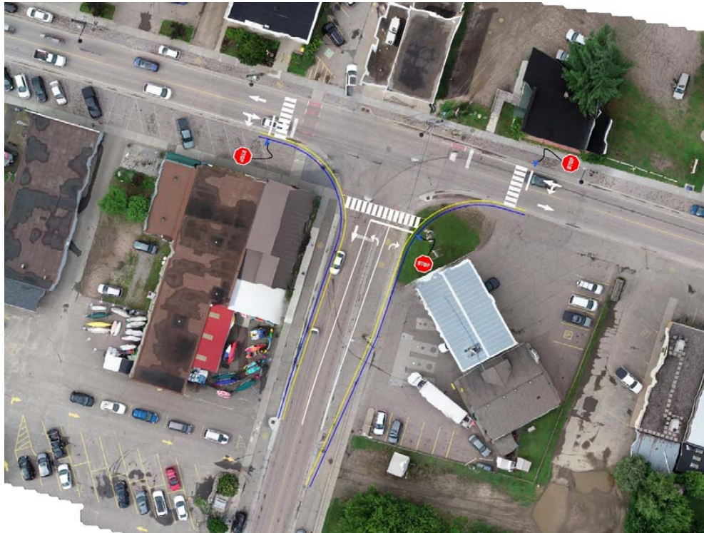
Figure 6.3 Layout Option 1: Addition of Right Turning Short Lane on South Approach
