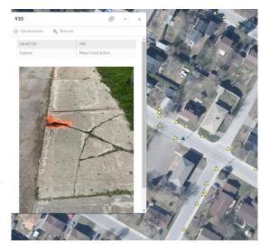
that exceed 2cm. In the past, they have generated public facing maps to send to a sidewalk grinding company with data points for just the repairs within their scope of work. They are piloting a separate quick capture app that allows workers to log when a repair is complete with a geolocated photo.
